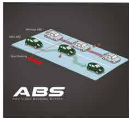
ANTI-LOCK BRAKING SYSTEM (ABS) ABS improves vehicle control by preventing wheels from locking in case of sudden braking.
