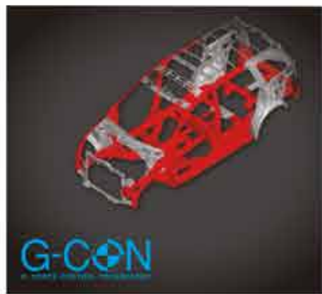
G-CON + ACE Honda's advanced safety technology distributes collision force across the vehicle to minimize injury.
